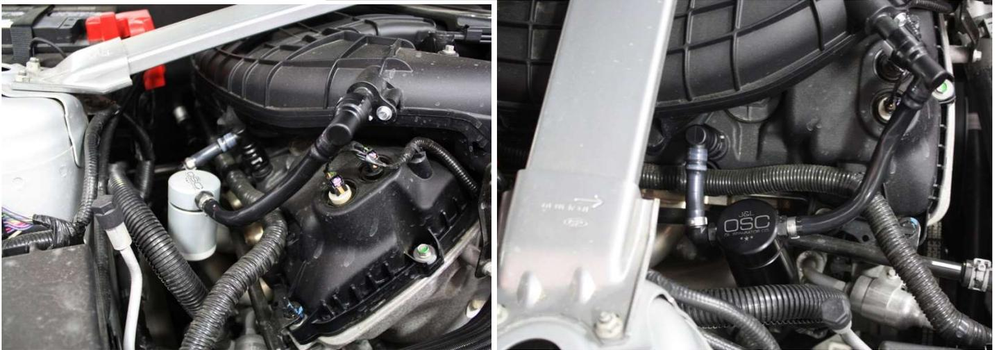
To properly clean the filter in the Oil Separator, spray any degreaser or solvent through it and let it air dry. Clean it every 10,000 miles.
